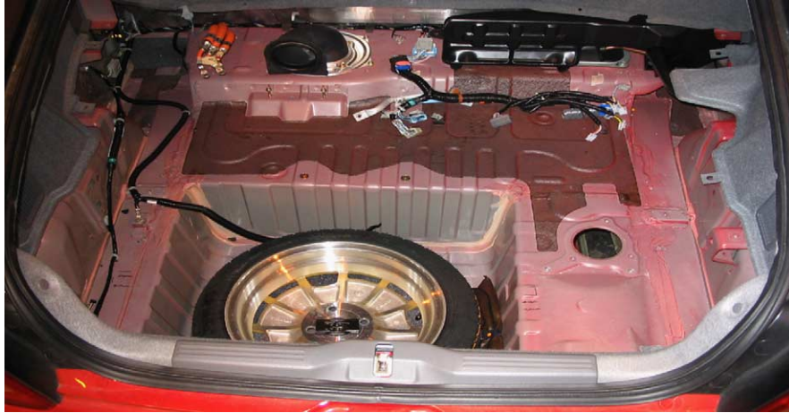
Fig. 1. Rear of Insight with Ni–MH battery and motor control module removed.
