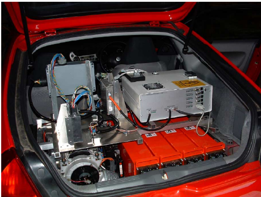
Fig. 5. Data logger and system controls in position.
