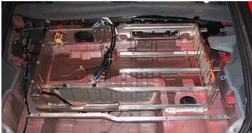
Fig. 2. Support frame for the lead–acid battery.
