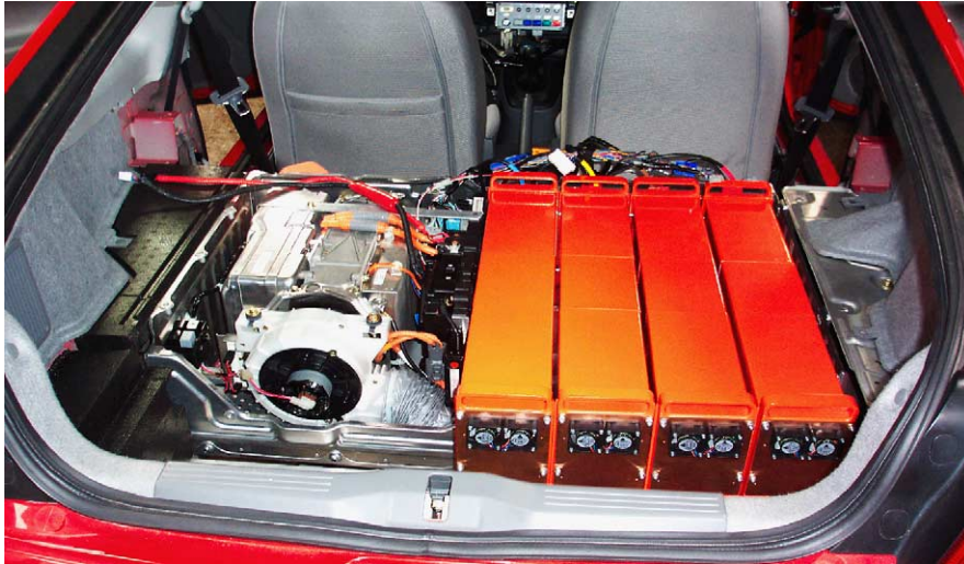
Fig. 4. RHOLAB lead–acid battery in position.
