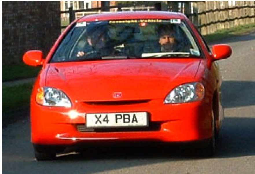
Fig. 6. RHOLAB Insight under road test with its lead–acid battery.
